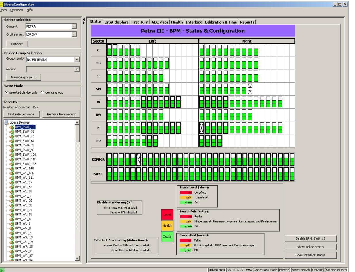
Libera Configurator: Status, Clock, Interlock, Overview and data display (All in One), allow experts to perform the initial setup as well as any general maintenance tasks
