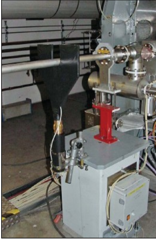
Fig. 23: Scintillator BLMs at FLASH (DESY); Left: Surrounding the beam pipe; Right: Long scintillator along an undulator. Courtesy L. Fröhlich, DESY.
