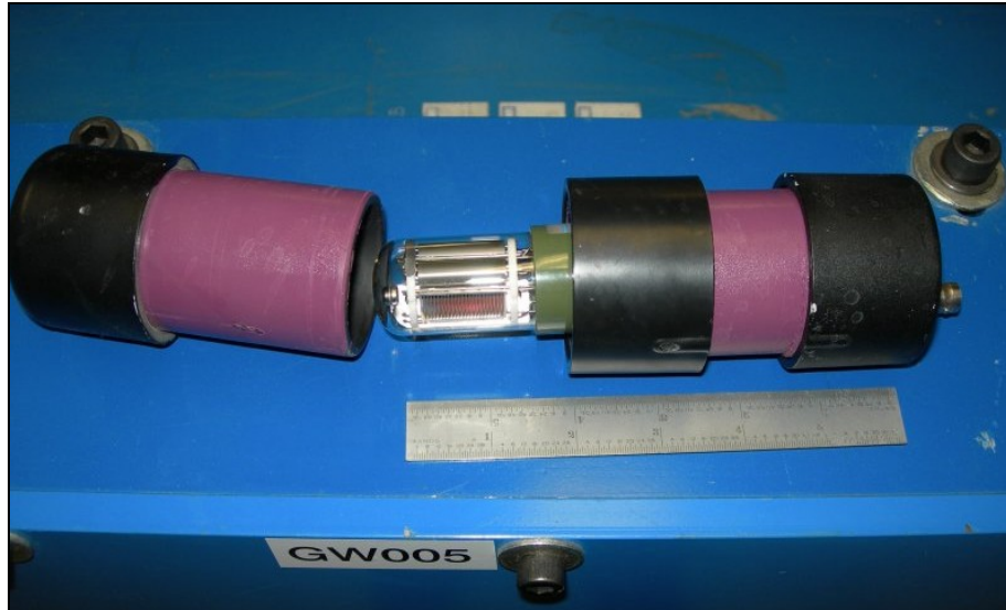
Fig. 25: The simple CEBAF Cherenkov BLMs. Courtesy K. Jordan.
