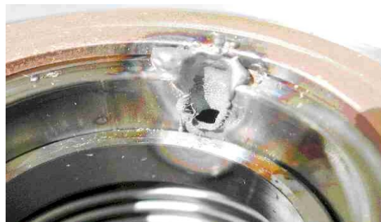
Fig. 6: Both figures show serious damage to vacuum components in the Tevatron [8] (left) and ELBE [9] (right) due to direct beam impact. In both cases no BLM system was available at the time.
