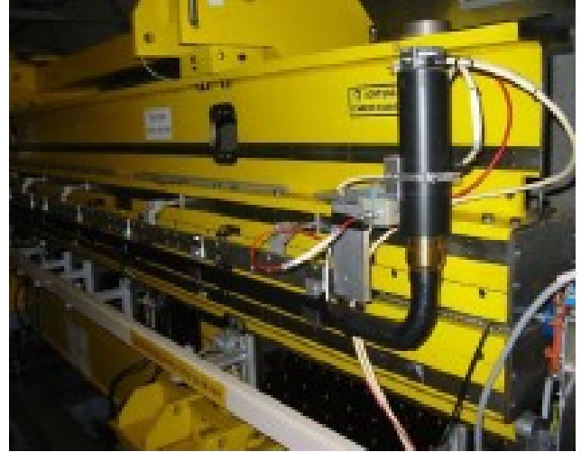
Fig. 23: Scintillator BLMs at FLASH (DESY); Left: Surrounding the beam pipe; Right: Long scintillator along an undulator. Courtesy L. Fröhlich, DESY.
