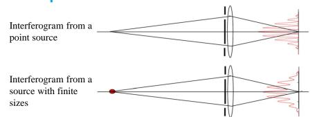
Formula for interferogram fitting is below. In this formula a denotes half of slit width,  $\lambda$  – observed wavelength, R – distance between back principal point of lens and image, y – coordinate, D – distance between slits. From this formula one can define  $\gamma$  and then  $\sigma$
