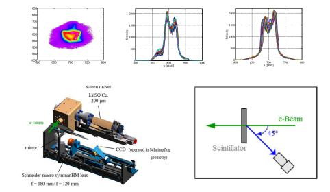
The main idea of where it comes from is a scintillator nonproportionality. The meaning of the effect is a nonlinear dependence of a scintillator light yield on an energy deposited in it by a particle. In other words the higher deposited energy the more e-h are created, and the higher e-h density the more possibility of them to "quench" (recombine nonradiatively).
