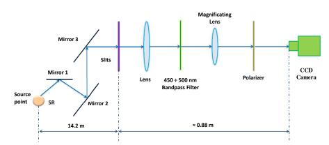
In figure 1 schematic of the new one interferometer is shown. Synchrotron light generated by electron beam in bending magnet and extracted from a tunnel by system of mirrors passes slits and the optical system and then comes to CCD camera.
