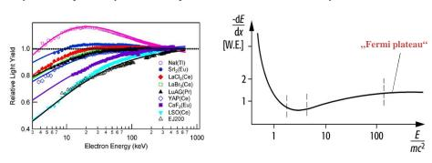
In our case the deposited energy of one electron isn't high enough (Fermi plateau) but we have high density of electrons in a beam ( $N_e \approx 3*10^9$  with Q=500 pC). Therefore when electrons are very close to each other they also can produce high density of e-h leading to quenching effect
