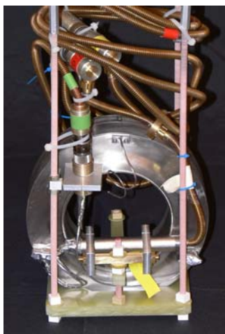
Fig. 4. Nb pick-up coil prepared for preliminary tests at 4.2 K in a liquid helium wide-neck cryostat.
