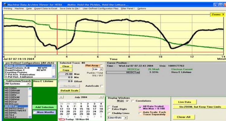
Figure 3: Archive data from HERA-e. Two short lifetime breakdowns are shown. The calculated lifetime shows a very slow response.
