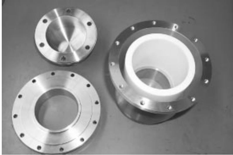
Figure 39: Dismantled absorber cavity.
