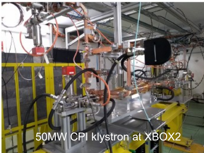
FIG. 29. The PolariX TDS installed in the XBOX2 test stand.
