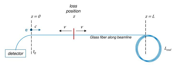
Timing of signal from loss at position z (from beginning of fiber in beamline)
