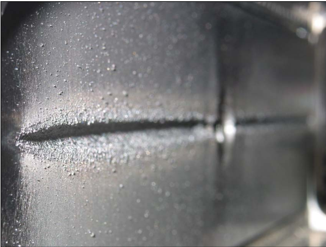
Fig 2, 3: 5 mm groove in the HERA proton collimator detected in 2003 after many years of operation. Courtesy of Mike Seidel, DESY.
