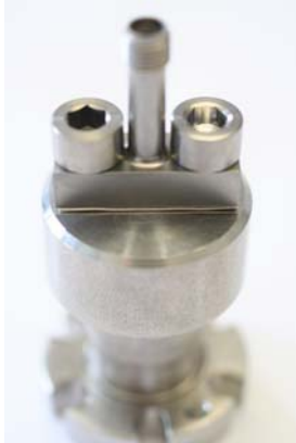
Fig. 9: Meggitt flange feedthrough mounted to the test adapter flange
