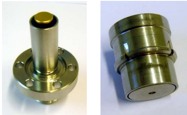
Fig. 14: These two pictures show different tested feedthrough from PMB, France. The left shows a gold plated stainless steel button with molybdenum conductor brazed to AL_2O_3 ceramic insulator. Usable directly mounting with the BPM body. The design is based on a
