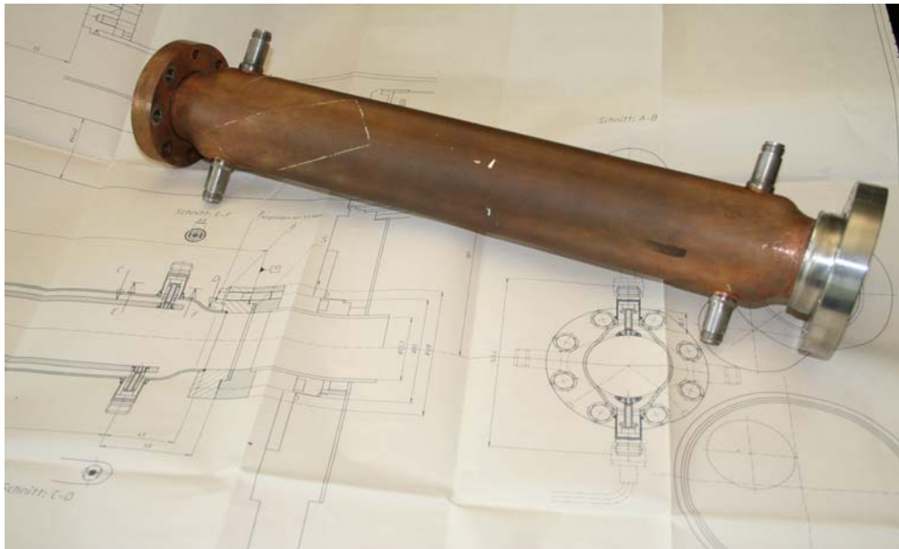
Fig. 3: Photo of a cold HERA proton BPM and its manufacturing drawing
