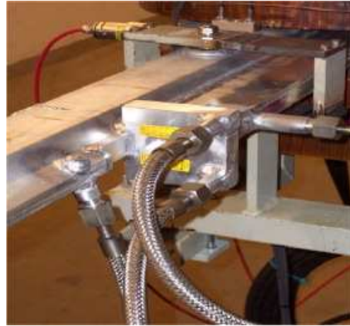
Figure 1: New exit window for Compton photons
